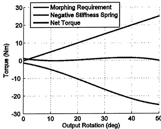
**Torque versus deflection for example system, showing the near zero net torque resulting from integration of a negative stiffness spring system**
