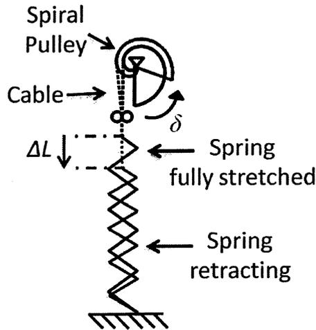
**Schematic of spiral spooling pulley and driving spring**
