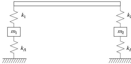
Figure 1. Two-bearing rotor.
