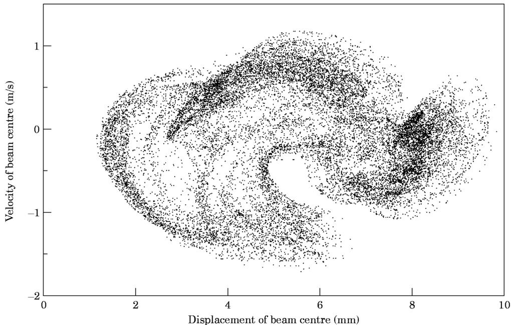
Figure 6. Poincaré map for the pinned beam with 16 d.o.f.
