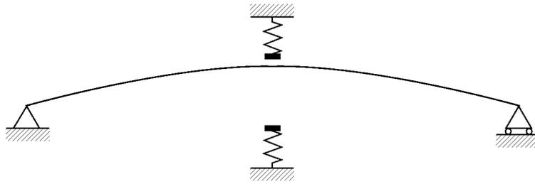
Figure 5. The pinned beam example (16-degrees-of-freedom). Flexural rigidity  $EI = 7.8750 \text{ N m}^2$ ; mass/unit length =  $0.4050 \text{ kg/m}$ ; beam length =  $1 \text{ m}$ ; proportional damping  $\mathbf{C} = \alpha\mathbf{M} + \beta\mathbf{K}$ ,  $\alpha = 5$ ,  $\beta = 10^{-5}$ ; discrete spring constant =  $20 \text{ kN/m}$ .
