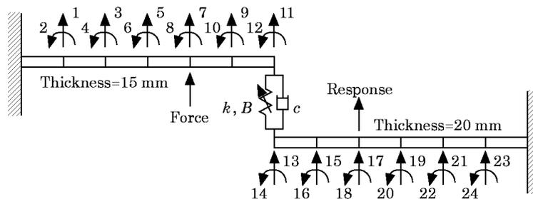
Figure 1. The twin cantilever beam example (24-degrees-of-freedom).  $k = 10 \text{ kN/m}$ ,  $B = 2 \text{ MN/m}^3$ ,  $c = 10 \text{ Ns/m}$ ,  $E = 70 \text{ GN/m}^2$ ,  $\rho = 2700 \text{ kg/m}^3$ .
