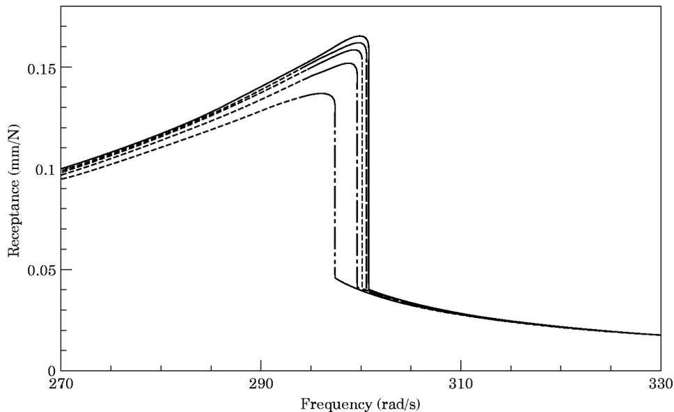
Figure 3. Results of reduction to modal co-ordinates for the twin cantilever beam example; the effect of the number of modes retained on the receptance near the second resonance. —, No reduction; ----, 7 modes; - · - · -, 6 modes; - - - - -, 5 modes; - · - · -, 4 modes.
