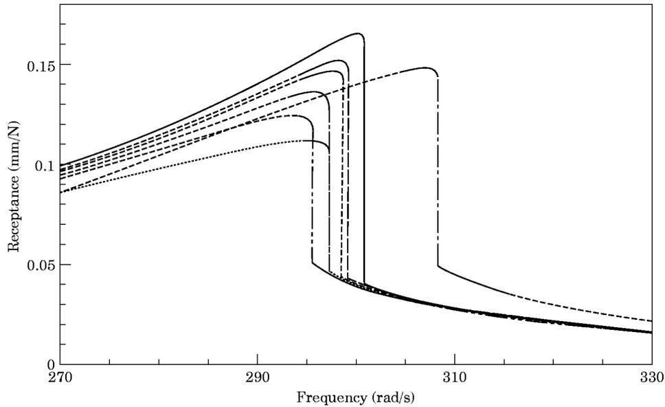
Figure 2. Results of IRS reduction for the twin cantilever beam example; the effect of the choice of master d.o.f. on the receptance near the second resonance. —, No reduction. D.o.f.: ----, 11, 12, 13, 14; ·····, 7, 11, 13, 17; - · - · - ·, 5, 9, 15, 19; - - - - -, 5, 6, 19, 20; ·····, 5, 6, 11, 12; ———, 1, 2, 3, 4.
