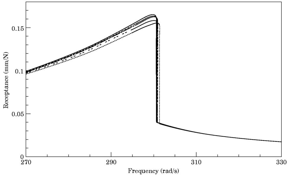
Figure 4. Results of reduction based on observability, controllability and balanced realizations for the twin cantilever beam example; the effect of the number of states retained on the receptance near the second resonance. Number of states: —, No reduction; ----, 14; - · - · - ·, 12; · · · · ·, 10; · · · · ·, 8.
