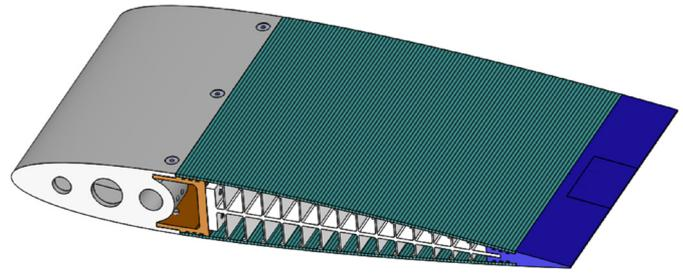
Fig. 1. Morphing airfoil with a compliant internal structure and flexible skin.
