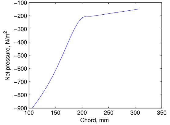
Fig. 5. Aerodynamic pressure loads on the upper skin.
