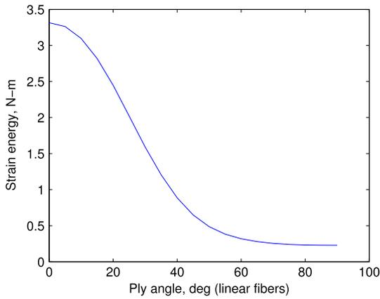
Fig. 8. Strain energy variation with respect to fiber angle (straight fibers).
