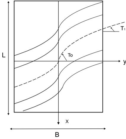
Fig. 7. Curved fiber paths in a composite plate.
