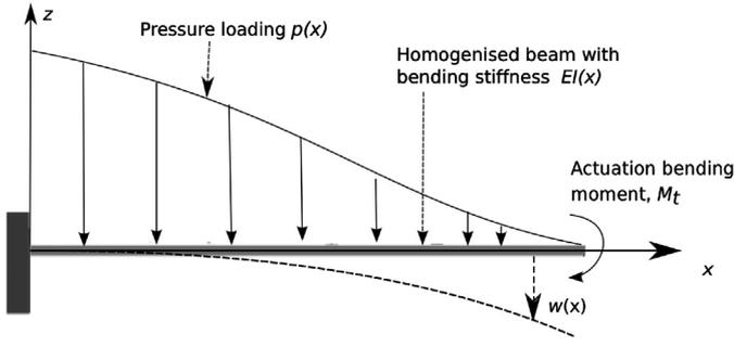
Fig. 3. Homogenized beam representation of the trailing edge aft of the D-spar.
