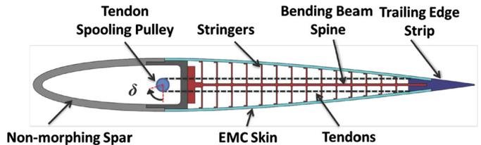
Fig. 2. FishBAC compliant structure.
