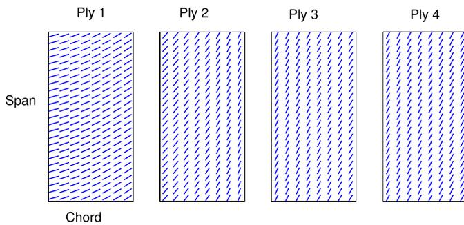
Fig. 10. Optimal curved fiber paths.
