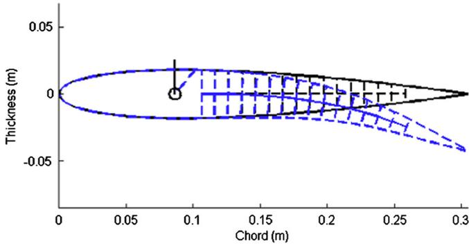
Fig. 4. Undeformed and morphed configuration of the airfoil.
