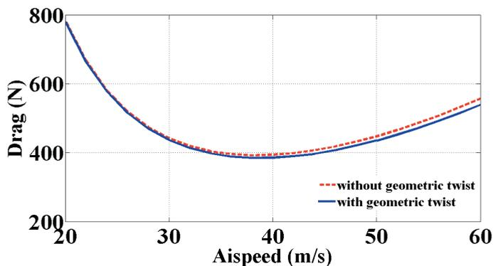
Figure 6. The drag polar of the flexible wing.
