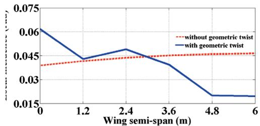
Figure 5. The spanwise incidence of the flexible wing.
