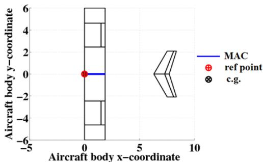
Figure 2. The geometry of the UAV in Tornado.
