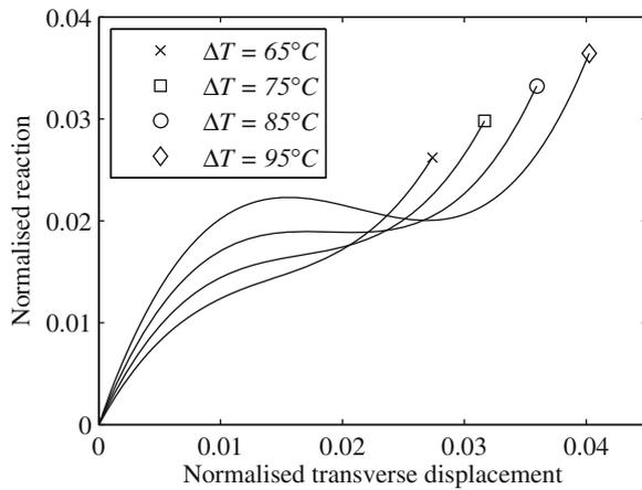
**Fig. 9.** The force-displacement response as a function of the initial thermal gradient,  $\Delta T$ .
