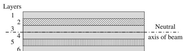
**Fig. 8.** A schematic of the composite beam with 6 layers. The coefficient of thermal expansion for layers 2 and 5 are different to that of the other layers.
