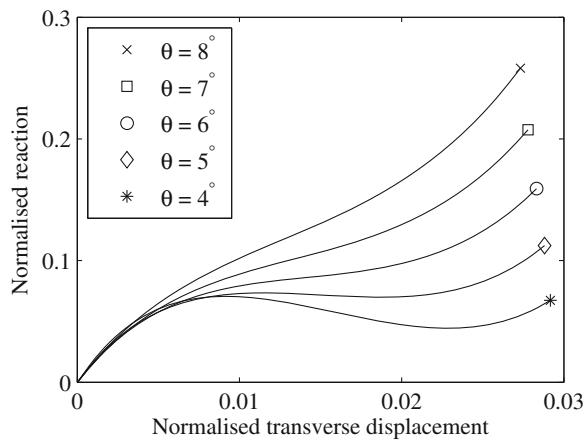
**Fig. 6.** Influence of prescribed rotation at the ends of the straight beam. The prescribed axial displacement is  $\delta = 0.001L$ .
