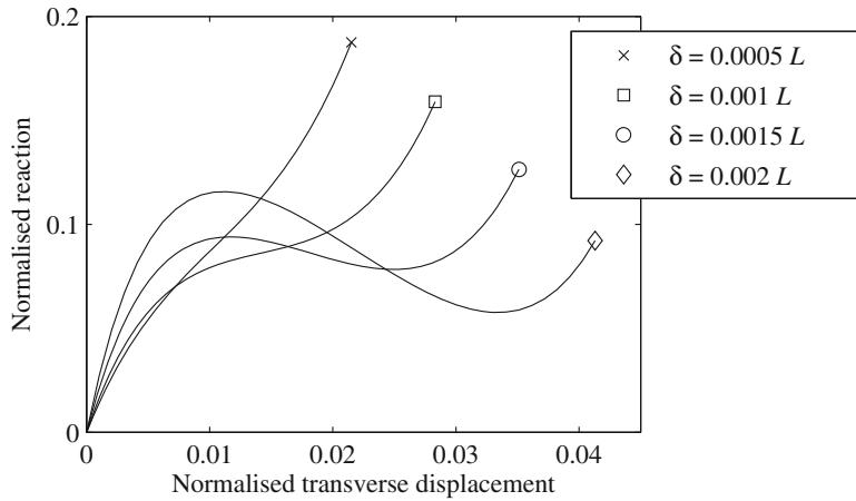
**Fig. 5.** Influence of prescribed axial displacement at the ends of the straight beam. The prescribed rotation is  $\theta = 6^\circ$ .
