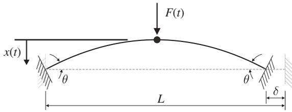
**Fig. 4.** Schematic of the beam subjected to prescribed axial displacement,  $\delta$ , and rotation,  $\theta$ , at both ends of the beam, followed by a prescribed transverse displacement at the beam centre. The beam is clamped once the prescribed axial displacement and rotation have been applied.
