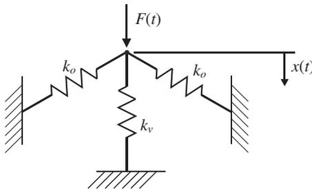
**Fig. 3.** Schematic representation of a mechanism with HSLDS characteristics: the oblique springs provide the necessary negative stiffness, whilst the vertical spring gives the positive stiffness.
