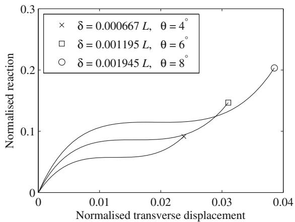
**Fig. 7.** Various choices of prescribed axial displacement and rotation that give a zero linear stiffness.
