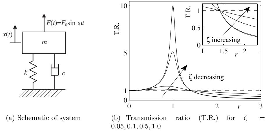
**Fig. 1.** Vibration isolation properties of a linear mount.
