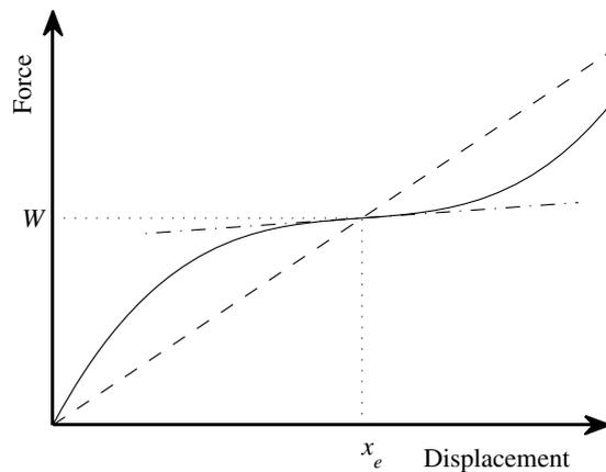
**Fig. 2.** The force-displacement characteristic of a linear (dashed) and a nonlinear (solid) spring. At equilibrium the static stiffness of the linear and nonlinear springs are equal, but the dynamic stiffness of the nonlinear spring (the slope given by the dot-dash line) is much smaller.  $x_e$  is the equilibrium displacement for the static load  $W$ .
