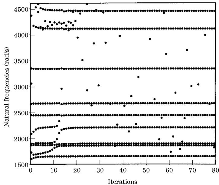
Figure 4. The convergence of the natural frequencies when using the dynamic IRS method with a large centre frequency  $\Omega = 3000$  rad/s.
