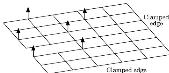
Figure 2. The finite element model of the slotted plate, showing the reduced co-ordinates.
