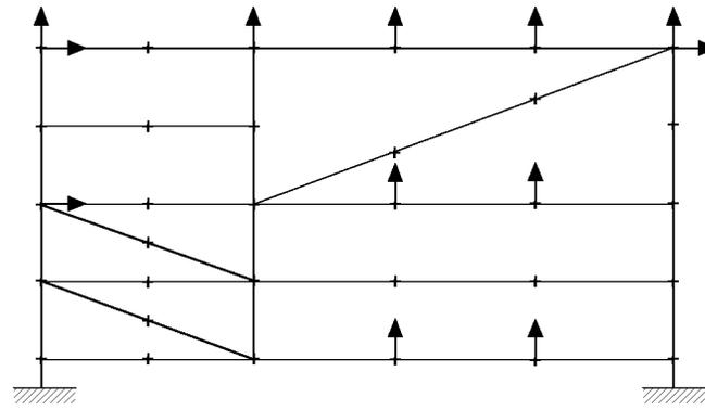
Figure 3. The frame example showing the node positions (+) and the reduced co-ordinates (arrows).
