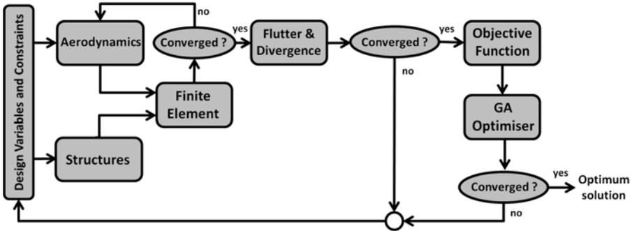
Figure 13. Flowchart and relational diagram of the MDO Suite.
