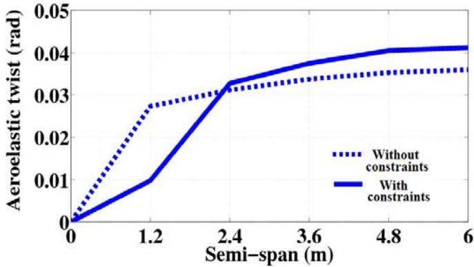
Figure 14. Spanwise aeroelastic twist to maximise rolling efficiency.
