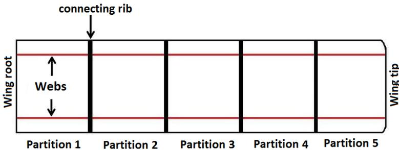
Figure 12. The multi-partition ATW concept without geometric pre-twist.
