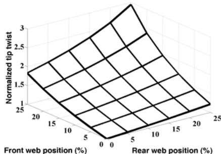
Figure 8. Variation of normalised tip twist.
