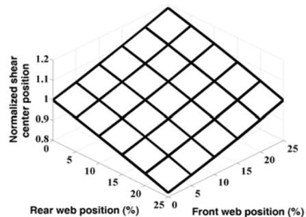
Figure 6. Variation of normalised shear centre position.
