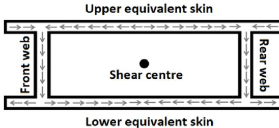
Figure 4. The shear flow in an equivalent wingbox section.
