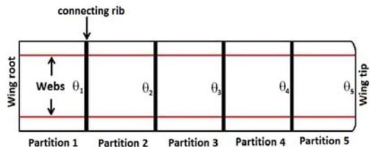
Figure 9. The multi-partition ATW concept with geometric pre-twist.
