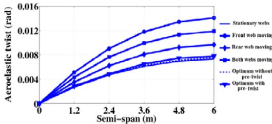
Figure 6. The spanwise aeroelastic twist of the ATW multi-partitions wing.
