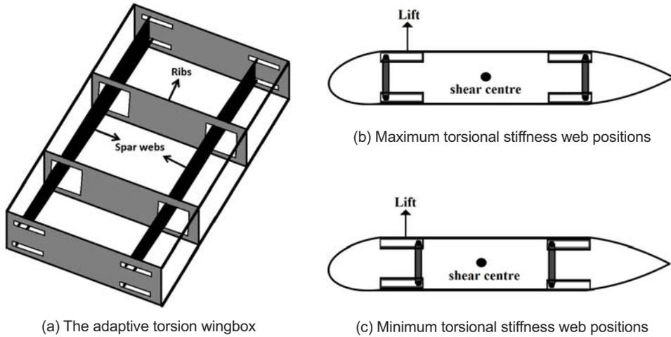
Figure 1. A conceptual sketch of the Adaptive Torsion Wing concept.
