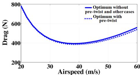
Figure 8. The drag polar of the ATW multi-partition wing.
