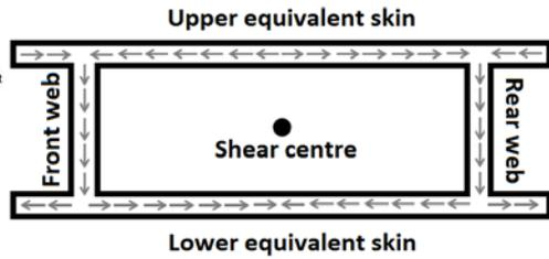
Figure 4. The shear flow in the equivalent rectangular wingbox section.
