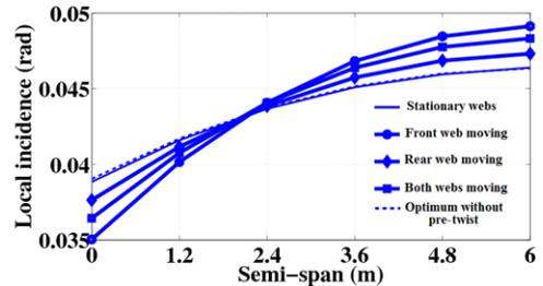
Figure 7. The spanwise incidence of the ATW multi-partition wing.
