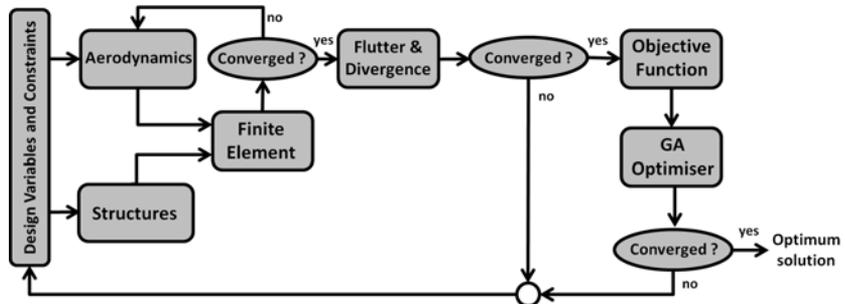
Figure 2. Flowchart and relational diagram of the MDO Suite.
