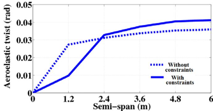
Figure 11. Spanwise aeroelastic twist over the ATW multi-partition wing to maximise rolling efficiency.
