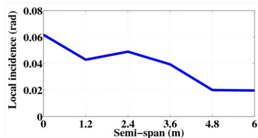
Figure 10. The spanwise local incidence of the multi-partition ATW with geometric pre-twist.
