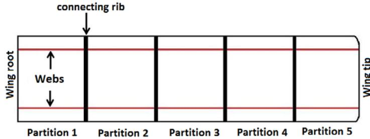
Figure 5. The multi-partition ATW concept without geometric pre-twist.
