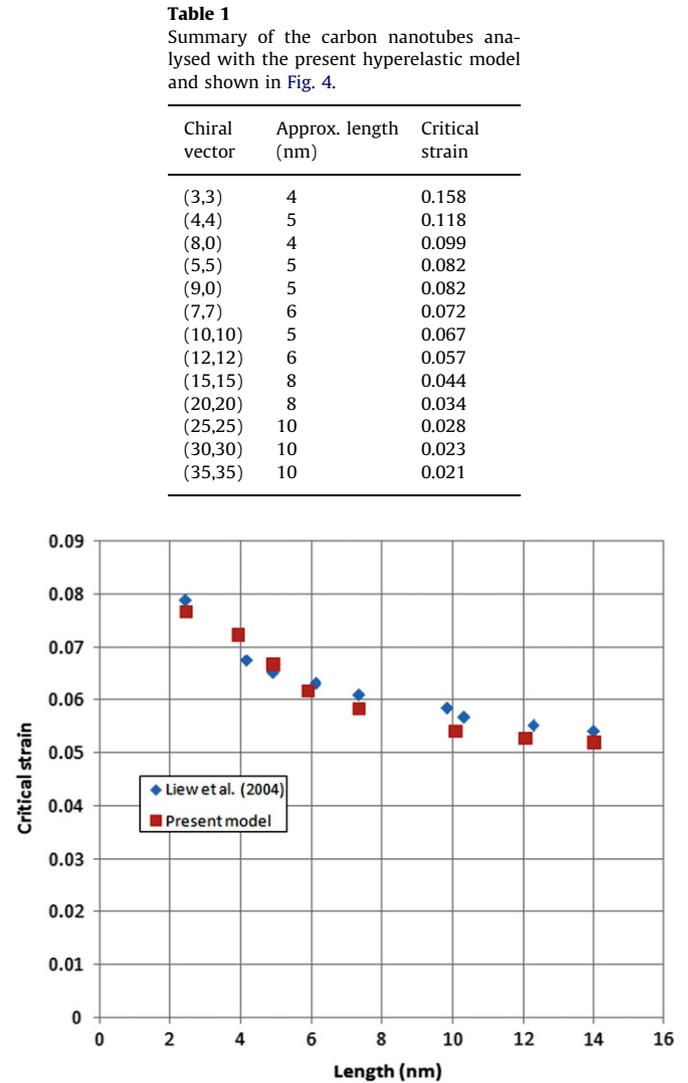
Fig. 5. Critical strains for (10,10) SWCNTs with different lengths.
