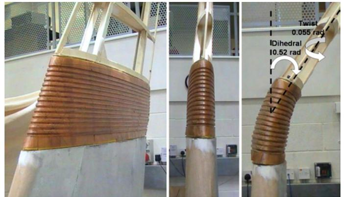
Figure 10. Rolled out and canted mechanical demonstrator (0.52 rad dihedral & 0.055 rad twist).
