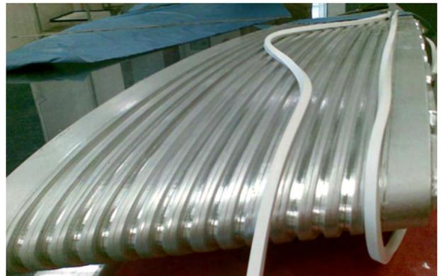
Figure 6. Aluminium mould for the corrugated skin.
