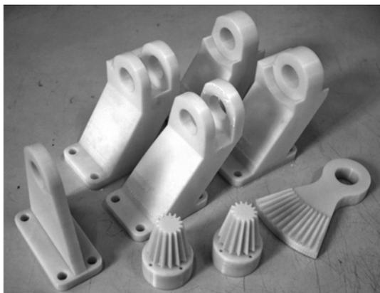
Figure 5. Servo-hinge linkage: rapid prototyping fabrication.
