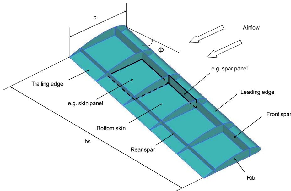
Figure 1: Wing structure layout for aeroelastic tailoring
