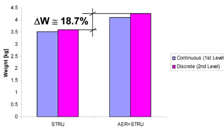
Figure 5: The weights of the optimum wing designs
